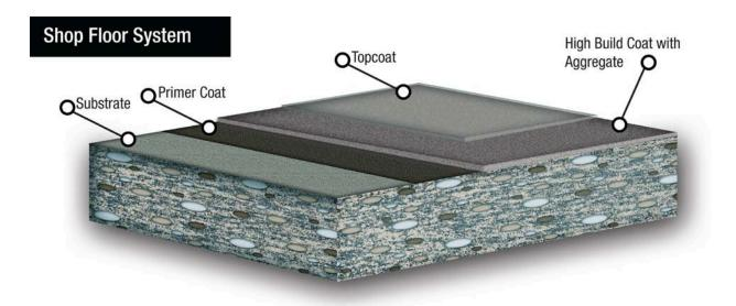
Shop Floor System is a high build, colored epoxy/urethane, high performance concrete coating system. It is used for environments requiring an attractive, high performance floor or when a concrete floor has sustained damage requiring a moderately thick surfacer with a slip resistant texture.
